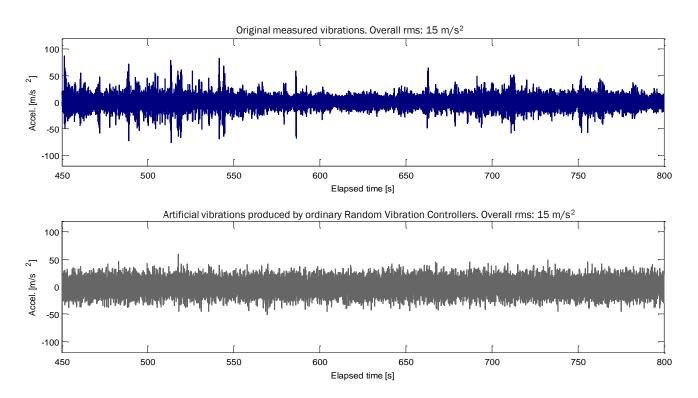
The Statistical Vibration Synthesizer (SVS) offers a practical solution to this problem. Based on years of University research, the Statistical Vibration Synthesizer converts your current random vibration test system into one that can reproduce the random fluctuations in rms that are so typical of vehicle vibrations.
