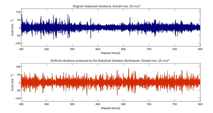
As shown above, the important advantage afforded by the SVS system is that it re-creates the occasional large excursions in vibration intensity that are clearly present in the original vibration record. Listen to the difference (signals played back at higher rates for audibility):
